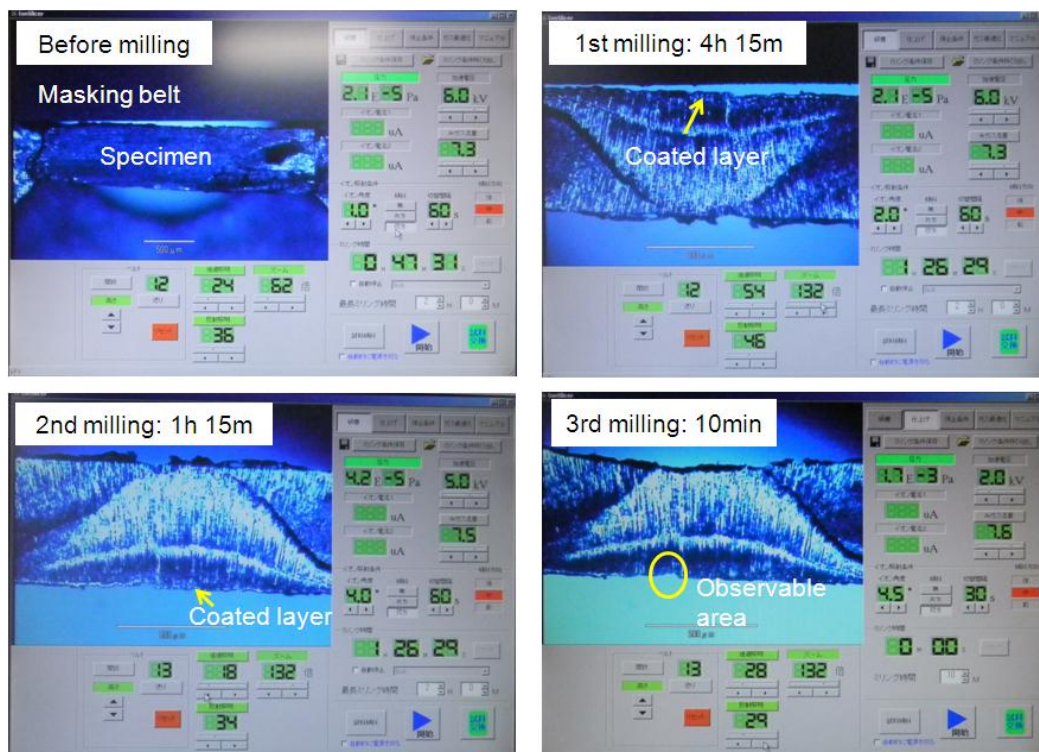
Figure 3.9. Typical thin (less than 1µm) “lagoon shaped” area produced by IS technique. The coated layer is indicated by the yellow arrow and an observable area is indicated by the yellow circle.
