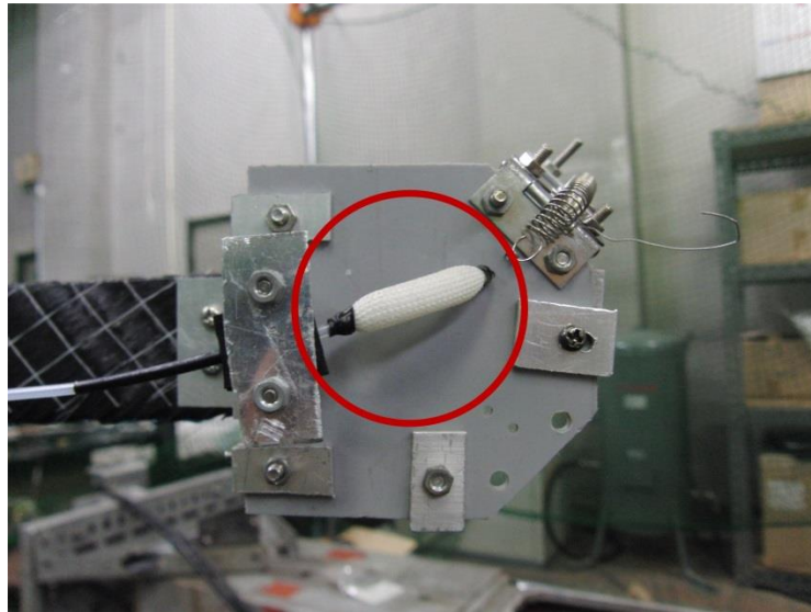
Fig. 5-5 Artificial muscle (SiktBw12PE30S)
