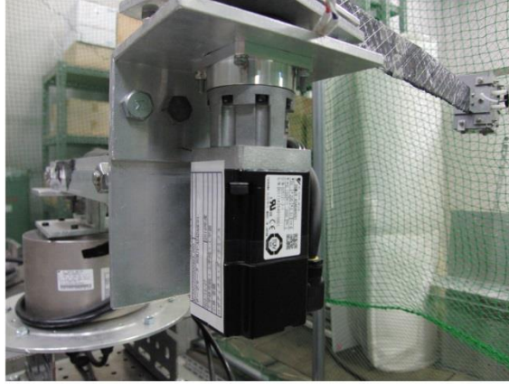
(a) AC servo motor SGMJVA5ADAHC01
