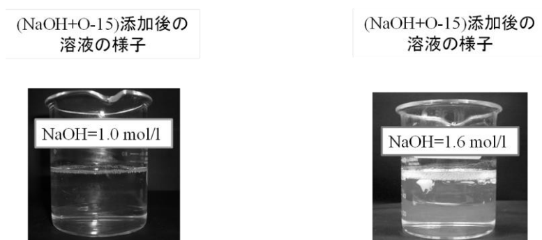
Figure 2.5 Appearance of synthesis gel after O-15 addition (NaOH concentration: (a) 1.0 or (b) 1.6 mol/L)
