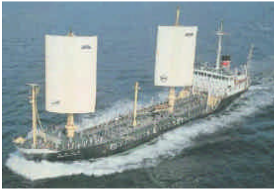
Fig.6 Sail-assisted tanker “Shin-Aitoku-Maru” (DWT: 1600, Sail area: 200m 2 )
