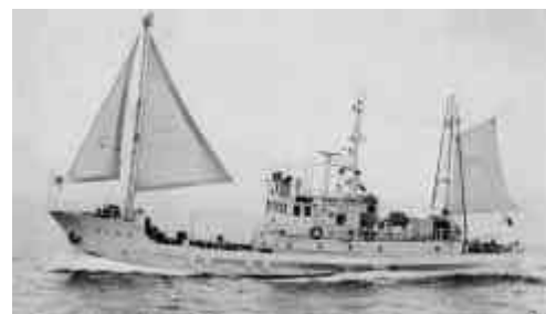
Fig.4 Sail-equipped fishing boat “Enoshima-Maru” (GT: 160, Sail area: 73m 2 )
