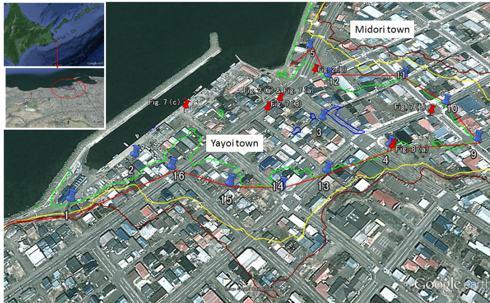
Fig. 10. Estimated runup limits (indicated by a red line) and surveyed sites at central Nemuro. Flood heights at sites 1 - 5 are listed in Table 1, and the locations of the runup limit sites are shown in Table 2. The locations where the photographs were taken (Fig. 2 a, b, Fig. 7 and Fig. 8 a) are indicated in the map. The ground elevation estimated from 5-m topographic data of GSI is indicated by the blue (1 m), green (2 m), yellow (4 m) and brown (6 m) contours.
