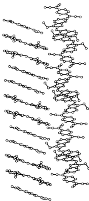
Figure1.3.5. The structural model of the 4,5,4',5'-Dibenzo-3,3'-diethyloxacyanine-TCNQ [19]. The cation component is \pi -conjugated and planar. Thus it can interact with another cation on one side and can also interact with TCNQ anion on the other side, leading to the formation of TCNQ anion dimer and DDAA type stack.
