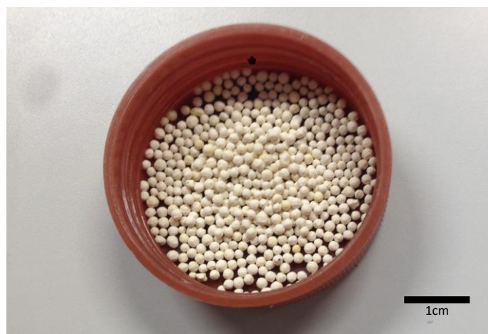
Fig. 4-1 Silver zeolite for the organic iodine filter.
