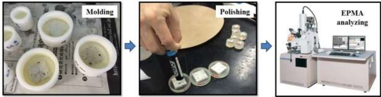
Fig. 3.4 Sample preparation for EPMA
