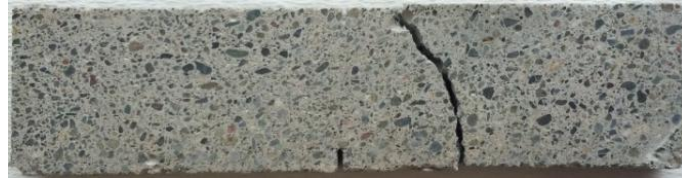
(b) For specimen with existing fire crack
