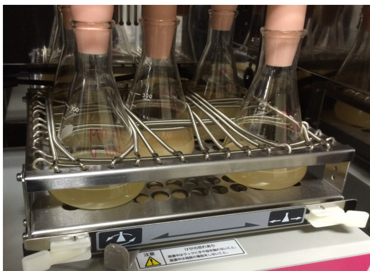
Fig.4.5: Culture solutions on the shaking table.
