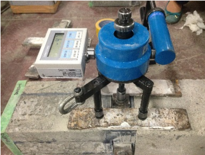
Fig. 6. Direct pull-off test setup
