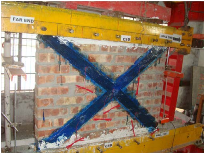
Fig. 7. Experimental setup of FRP reinforced masonry panel
