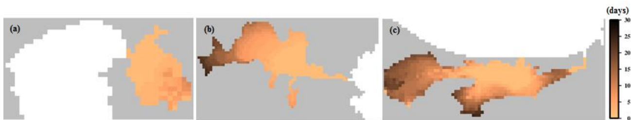
Fig. 5.4.3-4. Horizontal distribution of flushing time (days) at each grid in Akkeshi Lake, Hichirippu Lagoon, and Furen Lake simulated by the model.
