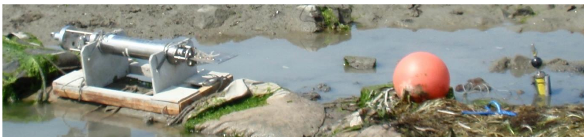
Fig. 2.2.2-1. Photograph of instruments (left: multiple-parameter probes, right: magnetic current meters) placed in the clam fishery ground.
