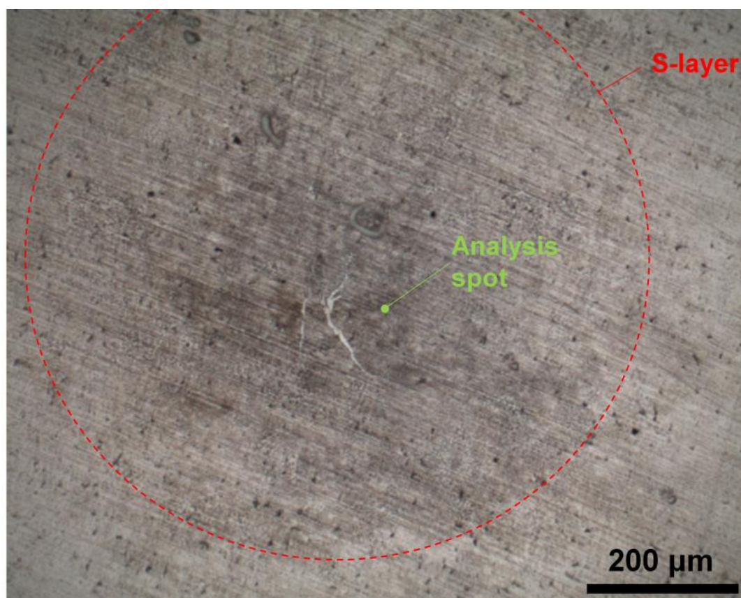
Figure 4.17 Optical microscopic image of the stainless steel surface after passivation at 0.9 V_{SSE} in a solution containing 2.8 \times 10^{-3} \text{ mol dm}^{-3} of \text{HS}^- by operation of LPIG.
