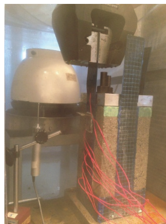
FIGURE 3: Specimen during the test under moisture condition.
