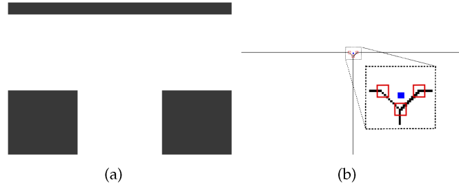
Figure 2. Node extraction from a skeleton map: (a) a map with obstacles and free space; (b) a corresponding skeleton map. Nearby nodes are clustered to form a single node.
