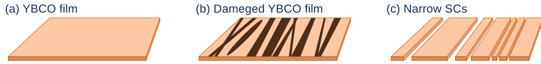
Figure 2.13: Schematic figures of thin films of a high- T_c superconductor as studied in Ref. [6]. They first fabricated thin films of a cuprate superconductor YBCO (a). After that, they irradiate heavy-ion beam on the films and create long but narrow holes (b). These samples can be regarded the collection of narrow superconductors (c).
