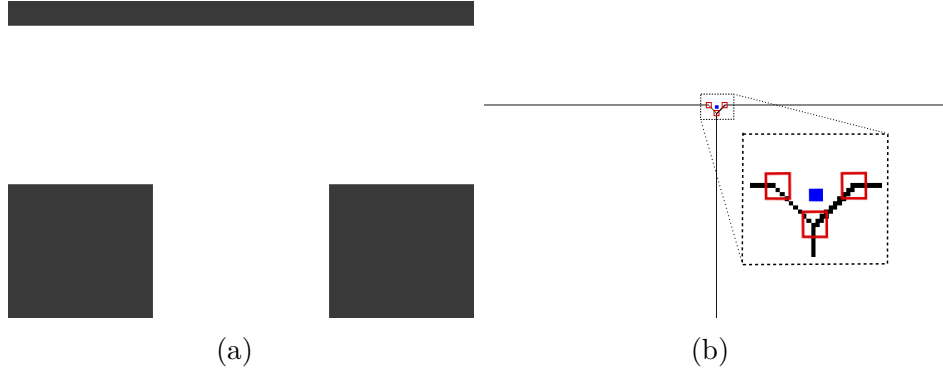
Fig. 2.2 Node extraction from skeleton map. (a) Map with obstacles and free space. (b) Corresponding skeleton map. Nearby nodes are clustered to form a single node.
