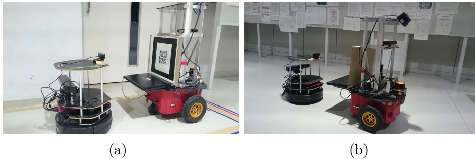
Fig. 6.9 Experiment 2. (a) Coupling between the two robots. (b) Turtlebot following P3DX through visual servoing.
