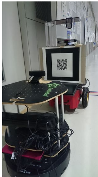
Fig. 6.1 QR code and camera system for coupling.
