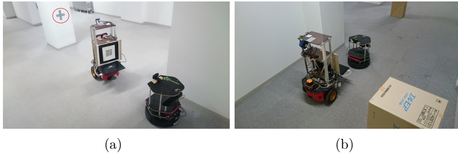
Fig. 6.6 Experiment 1. (a) Coupling between the two robots. (b) Turtlebot following P3DX through visual servoing.
