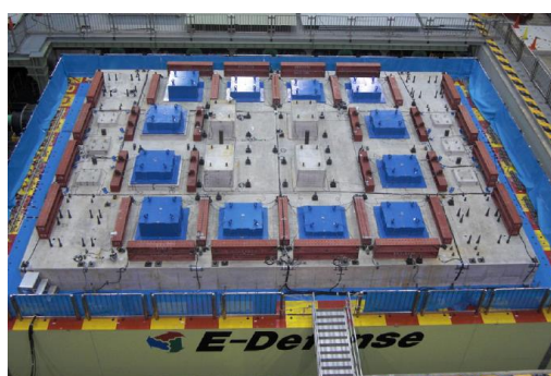
(c) 12 test bodies on the shaking table
