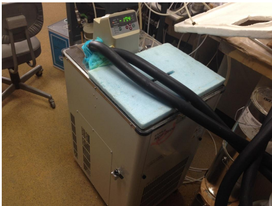
Figure 3-4 Refrigerating bath (EYELA NCB2600) for circulating low-temperature refrigerant in the triaxial apparatus
