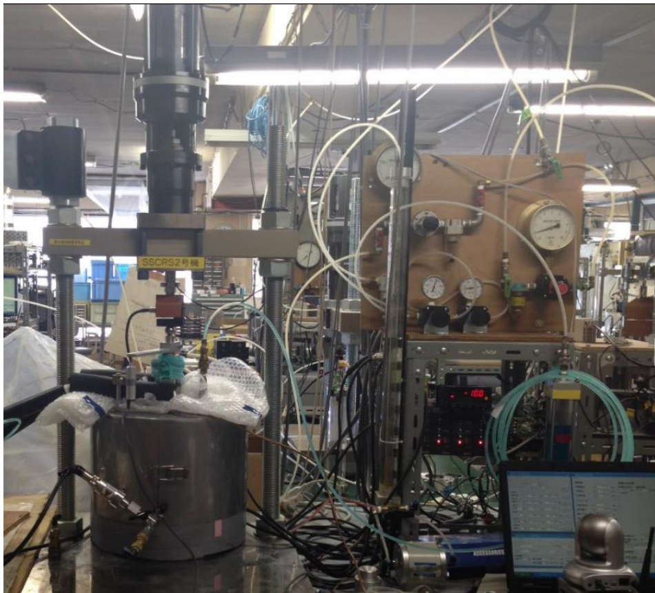
Figure 3-11 Image of the triaxial compression test on frozen soil at -10 °C
