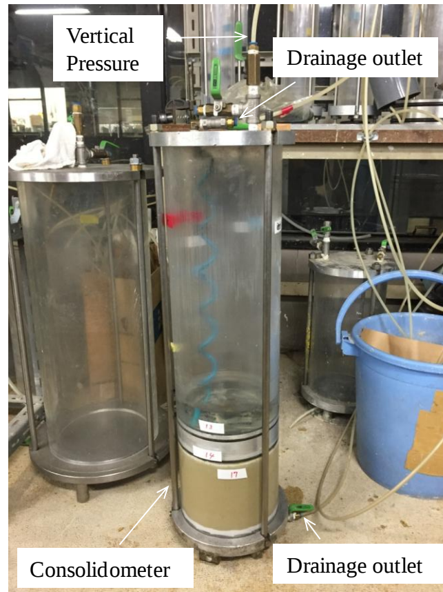
Figure 3-2 Sample under K_0 preconsolidation in a consolidometer (the inner diameter: 16.5cm.)
