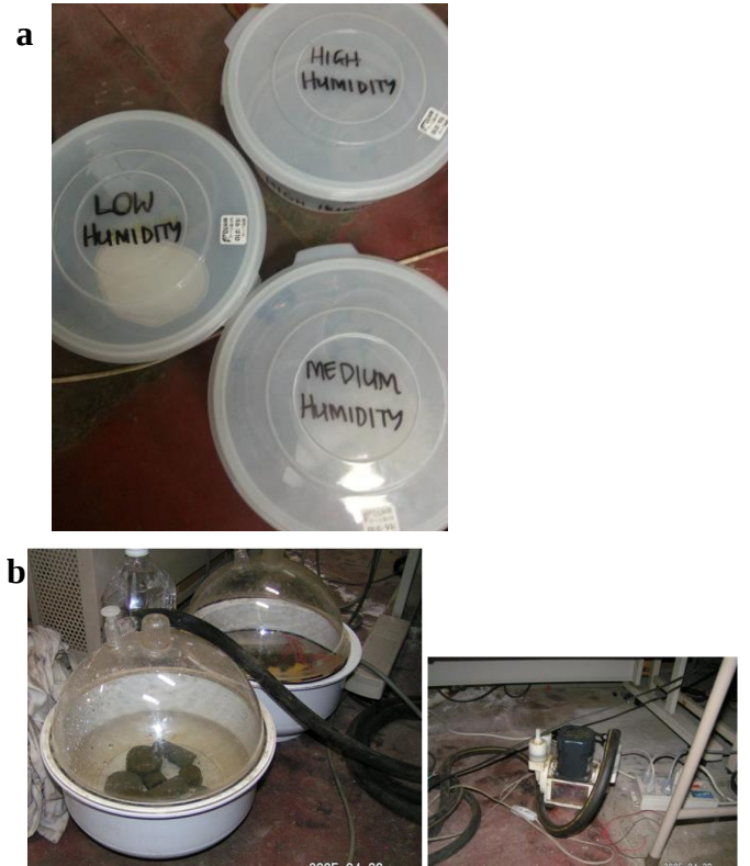
Fig. 9. (a) Air-tight containers with specimens in the laboratory, (b) Vacuum saturation of specimens
