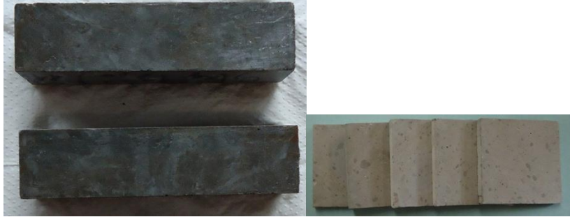
Figure 2.1 Cement paste specimen and paste disks using in migration cell.
