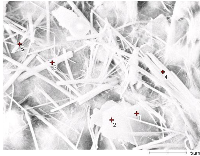
c) Ettringite (needles such as +3, +4 and +5) and Friedel's salt (hexagonal plates +1 and +2).
