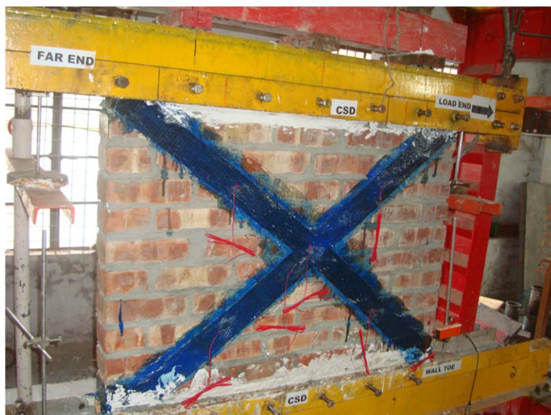
Fig. 5.13. Experimental setup of FRP reinforced masonry
