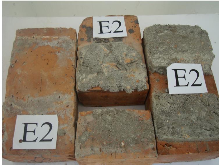
Fig. 3.9. Failure surface of a typical shear specimen
