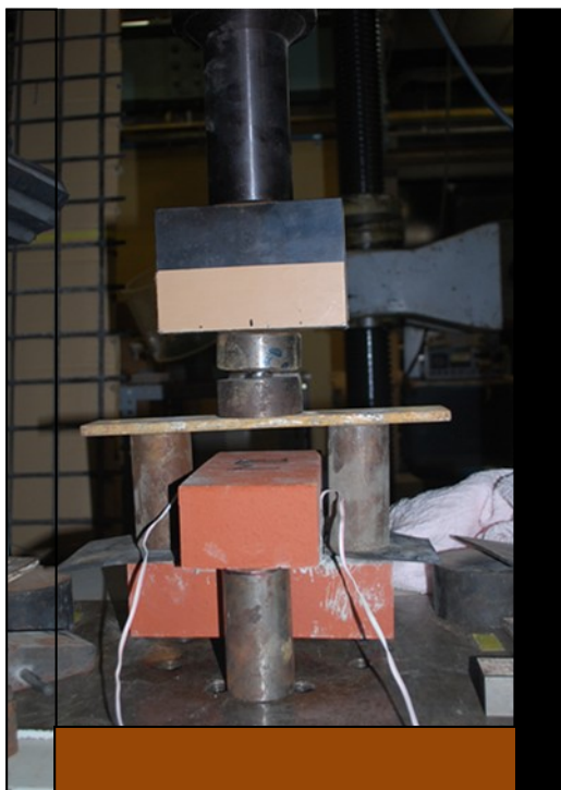
Fig. 3.14. Experimental setup of crossed-brick test
