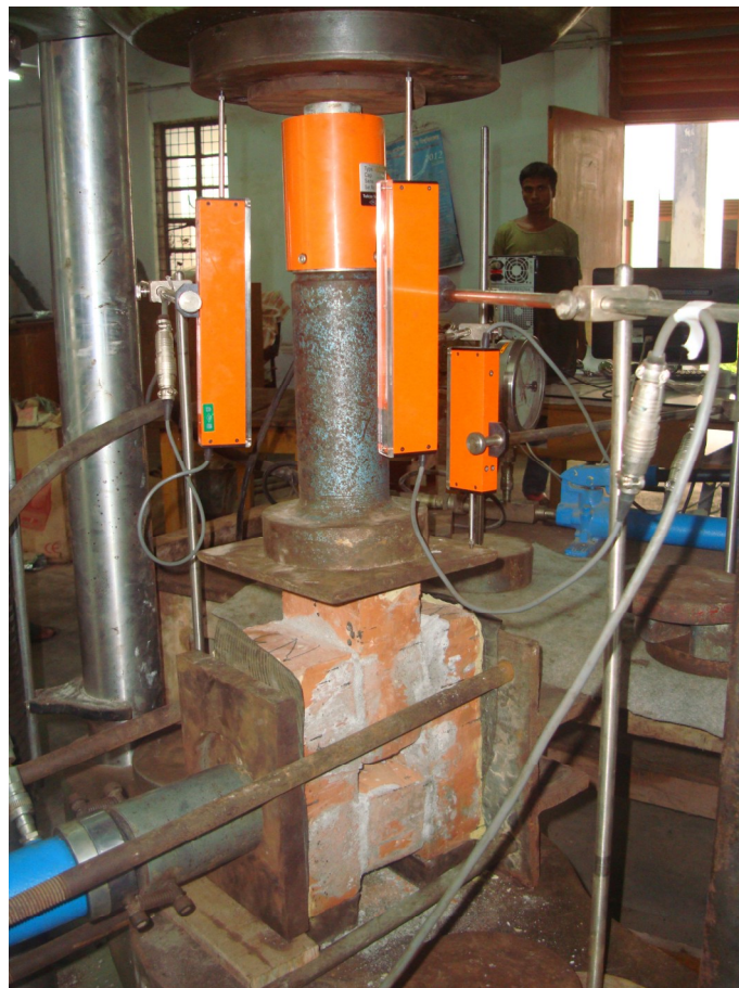
Fig. 3.4. Instrumentation and test setup of shear specimen
