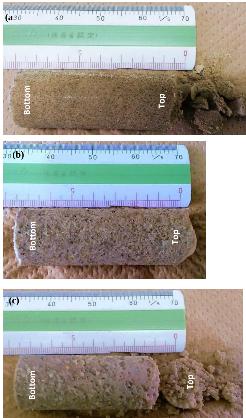
Fig. 4.23: Solidified sand test specimens (a) Toyoura (b) Mikawa and (c) Mizunami sand.
