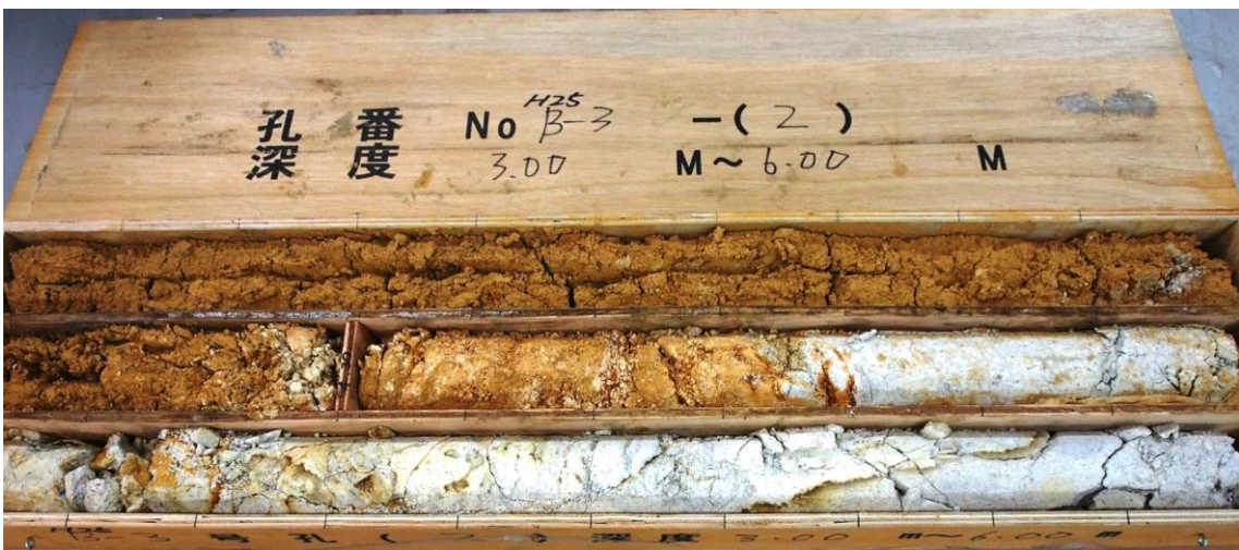
Figure 2.12 Core samples at depth 3 m to 6 m (Up to 4 m Talus sediments and after 4 m depth Andesite bedrock)
