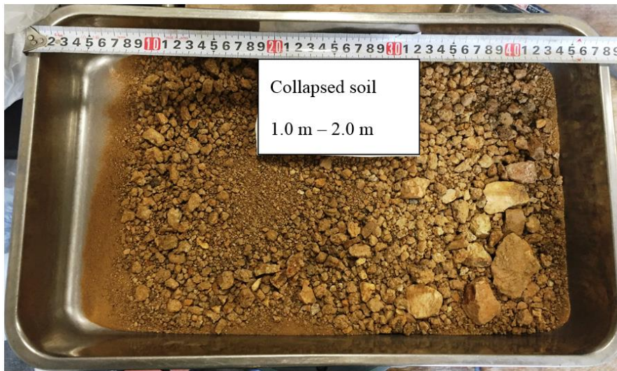
Figure 2.15 Picture showing collapsed soil at depths 1.0 m to 2.0 m
