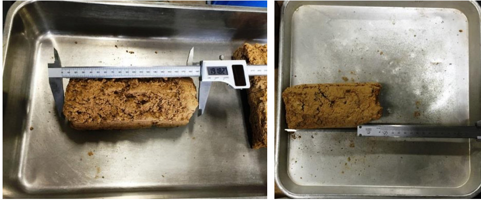
Figure 2.14 Measurement of length and diameter of selected cylindrical samples for dry density test
