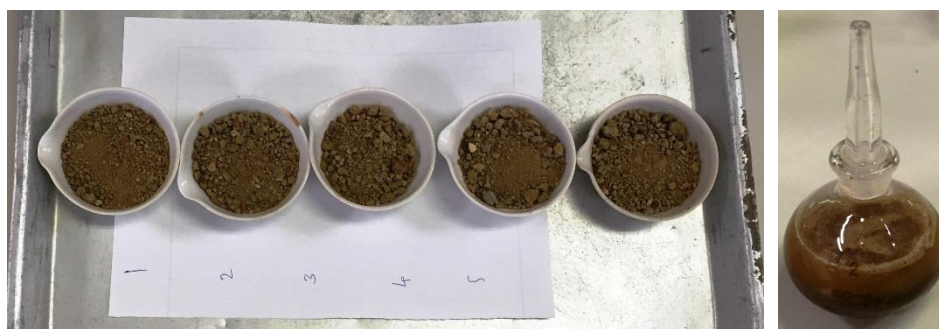
Figure 2.17 (a) Specimens used for solid density tests and (b) a view of a pycnometer filled with distilled water and soil specimen kept for reaching a steady room temperature
