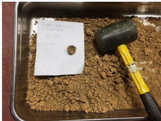
Figure 2.16 View of crushing of samples for soil density tests
