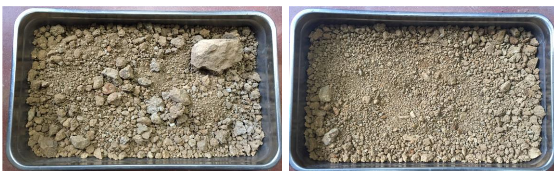
Figure 2.18 Photo showing collapsed soil from cores taken at depth 1.0 m to 2.0 m and cores taken at depths 3.0 m to 4.0 m
