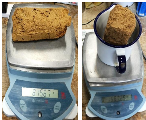
Figure 2.13 Mass measurements of cylindrical samples randomly selected at each 1 m depth for water content tests
