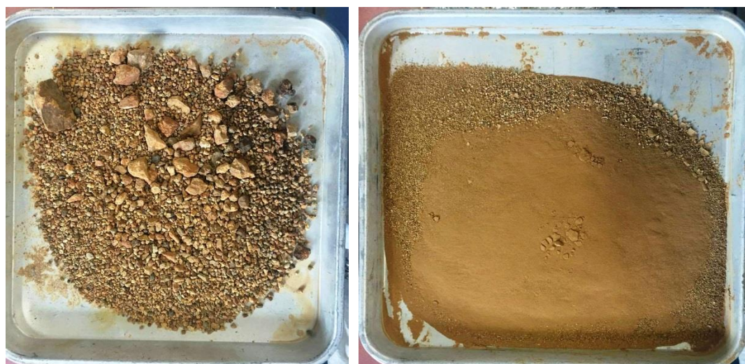
Figure 2.19 Photographs showing soil particles remained in (a) 2 mm sieve and (b) soil particles remained in 75 µm sieve (soil corresponding to core specimens at depth 3.0 m to 4.0 m)
