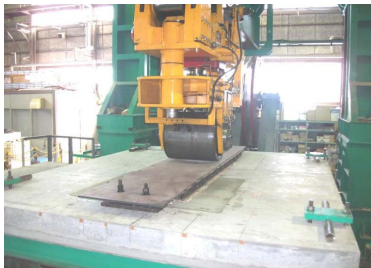
Figure 1.1 Experiment set-up for cyclic moving loads
