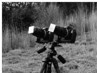
Fig. 1. (Top) Basic configuration of the \text{SO}_2 camera developed in the present study. (Bottom) \text{SO}_2 camera in field operation. Two CCDs are mounted alongside on a tripod.
