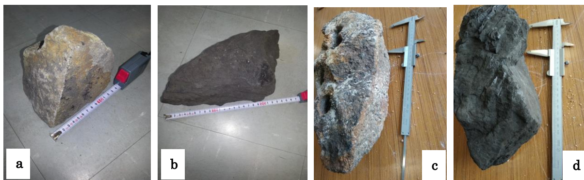
Fig. 1 Rock samples from Mchenga coal mine (a) arkose sandstone (b) fine-grained sandstone; and Kaziwiziwi coal mine (c) arkose sandstone (d) fine-grained sandstone
