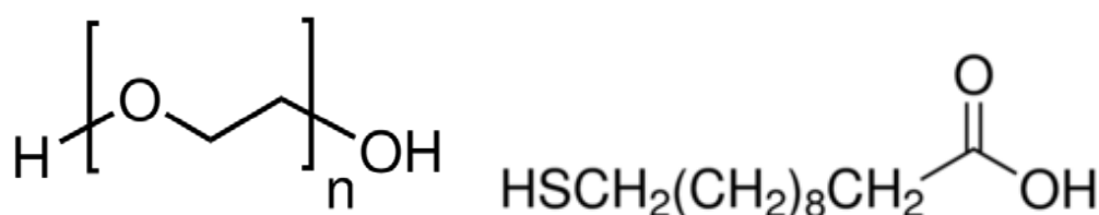
Figure 4.1. Molecular structure of polyethylene glycol (left) and of 11-mercaptoundecanoic acid (right).
