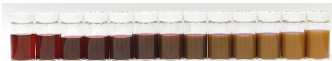
Figure 1.3 Illustration of the seeded growth of Au NPs, from 12 nm (left) to 120 nm in diameter (right), as described by Bastus et al. [111]
