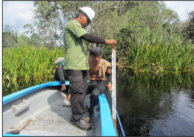
Figure 3.5 Flow rate measurements in the downstream end of Turip River (TR).
