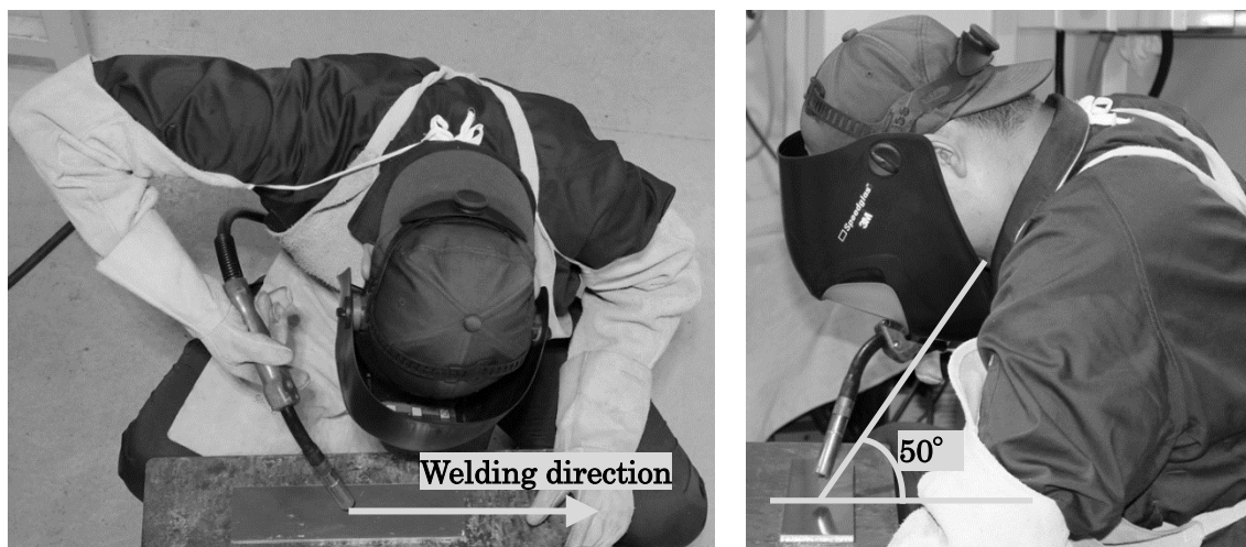
Figure 3.11 General welding position of GMAW at flat forehead welding
