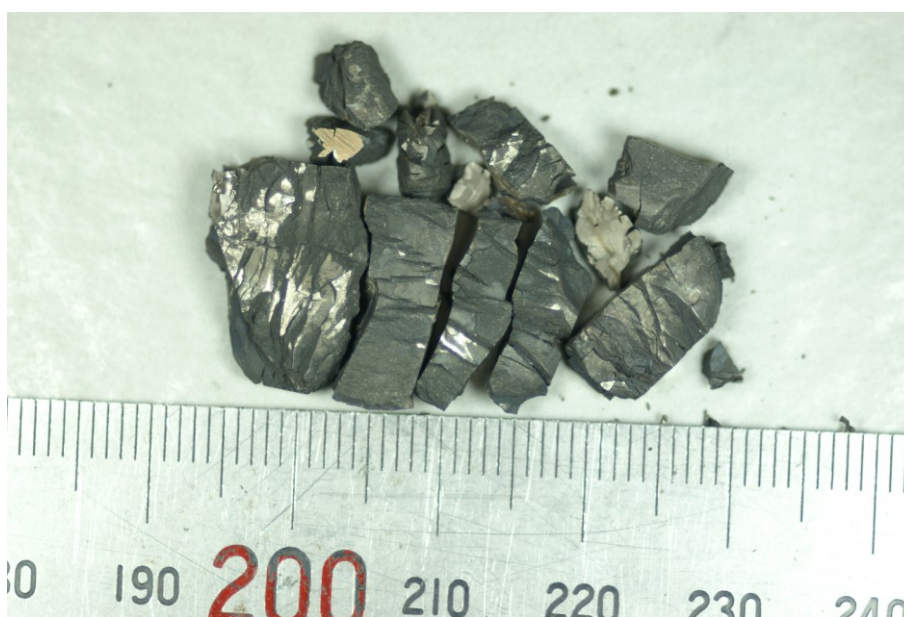
Fig. 3.3 The 15AlCrY sample after hot rolling at 1200 °C.
