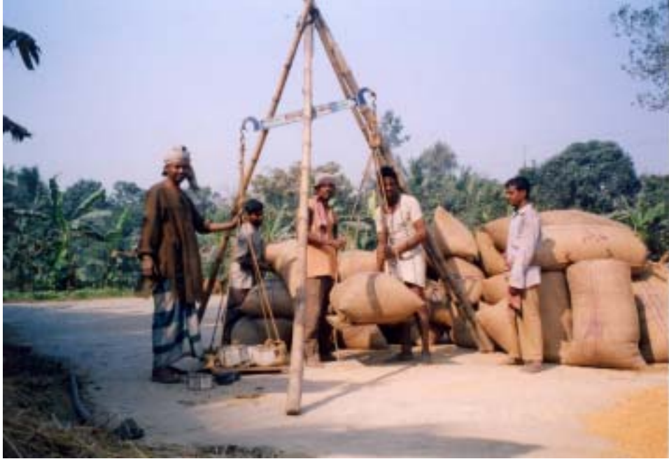
Fig. 6 A local-type balance used to measure the mass of paddy and husk
