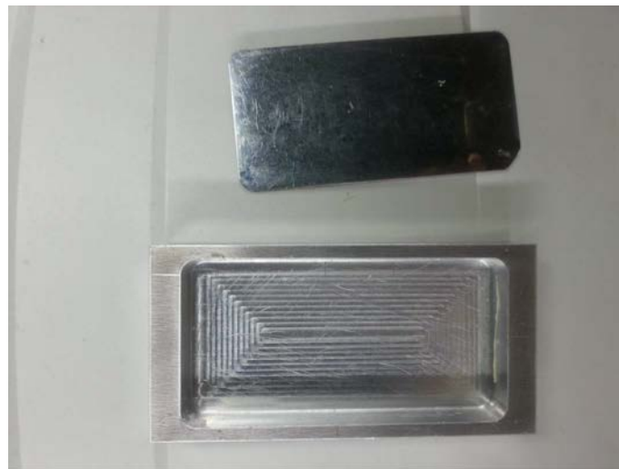
Fig. 2 Aluminum mold and stainless steel plate.
