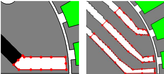
(a) Base model of IPM motor represented by a polygon (b) Base model of SynRM represented by polygons Fig.5 Shape optimization based on polygon morphing
