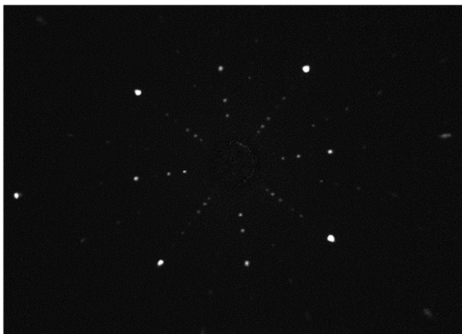
Fig. 4-6. A Laue image of \text{UAu}_2\text{Si}_2 single crystal grown by floating zone method. The c axis is oriented.
