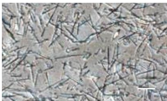
Figure 3.19 Micrographs of crystals composed of C6AC6 and various fatty acids (bar = 50 μm).
