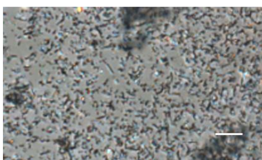
Figure 3.17 Micrographs of crystals composed of C2AC8 and various fatty acids
