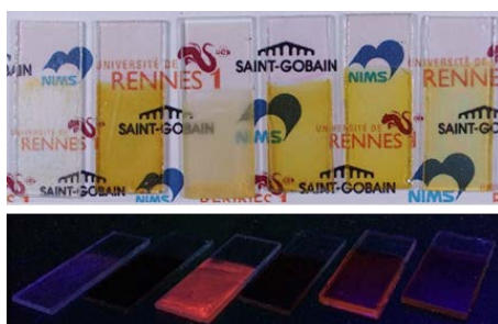
Figure 2.4. The \text{Mo}_6 cluster thin films deposited from (left to right) water, ethanol, 1-propanol, acetone and MEK solutions at 15 V for 20 s and from acetyl acetone solution at 50 V for 40 s (upper), respectively. Image of the luminescence of the cluster thin films irradiated at 324 nm wavelength (under).
