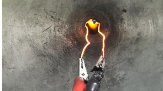
(b) Nichrome wire ignition during low oxidizer supply
