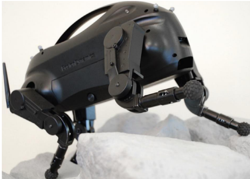
Figure 2.2: Boston Dynamics LittleDog research platform walking over an obstacle. Motion capture and Wi-Fi connectivity accessories have been added to enable remote visual servoing [4].
