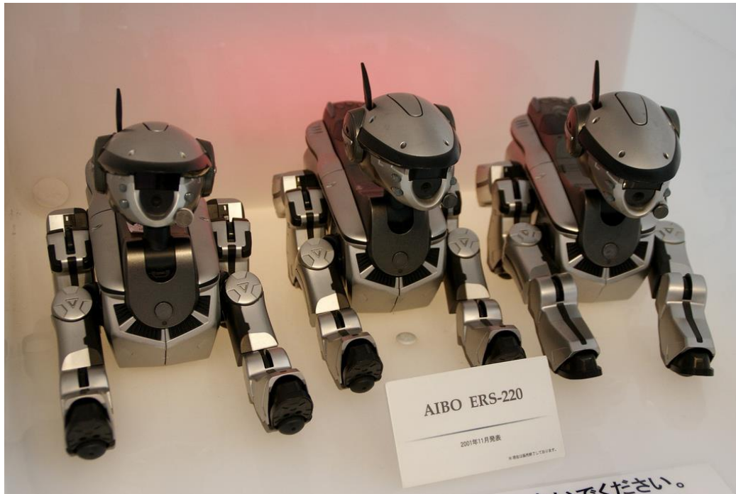
Figure 2.1: Second generation Sony Aibo with integrated camera and Wi-Fi connection [2]. Few platforms have had as much widespread use in robotics research as the Aibo line.
