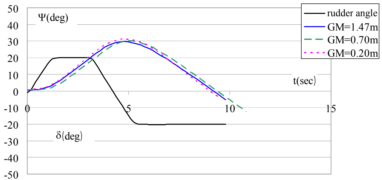
Fig.4.3(a) Comparison of 20^\circ - 20^\circ Z tests time history, between GM (135GT fisher boat, F_n=0.3 )
