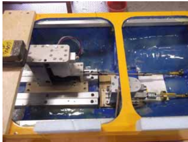
Fig.3.6 Setting of self-propulsion dynamometer for two axle Ferry
