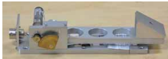
Fig.2.22 Elevator machine for prism
