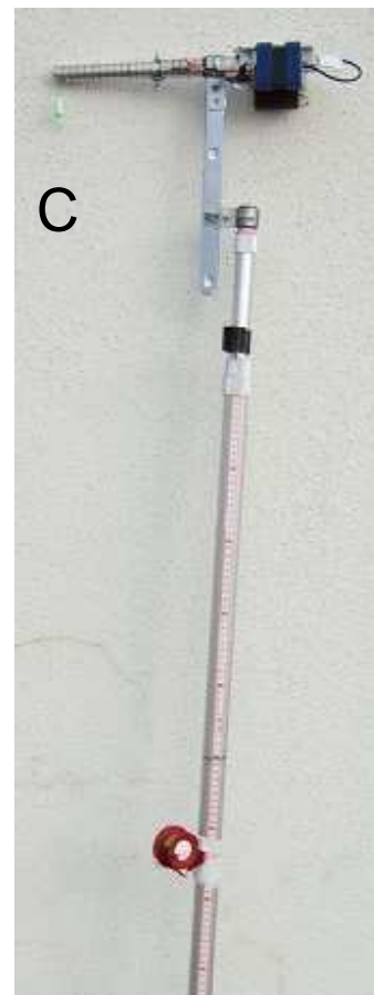
Photo 1 A cavity measurement system. A cavity viewer using a wireless CCD camera was originally developed by Matsuoka (2002; 2010).
