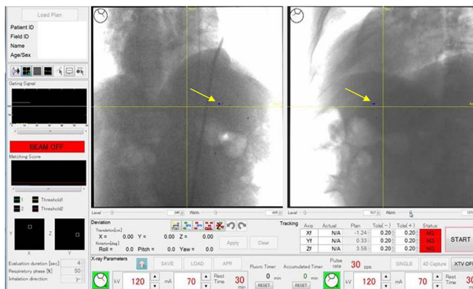
Fig. 2. Console display of the real-time-image gated proton beam therapy (RGPT) system for a patient with a liver tumor. Two sets of fluoroscopic images are shown with the projection of the planned position of the internal fiducial markers (arrows). The scanning pencil beam of protons is delivered only when the fiducial marker is within \pm 2 mm of the planned position. The rate of recording was 30 frames per second for this patient. Other parameters of the fluoroscopy are shown in the display. During the actual irradiation, the imaged area is collimated to reduce unnecessary X-ray exposure.
