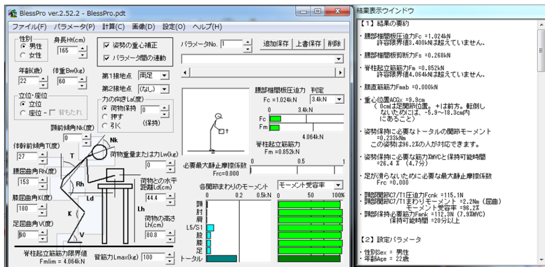
Fig. 1.2.3: A simple supporting software for redesigning working conditions to reduce low back load 「BlessPro」 [37]
