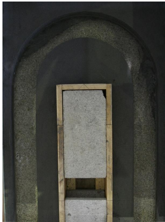
Figure 2.13: Snapshot taken after 16 hours of sediment equilibrium condition.
