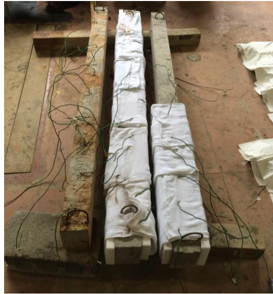
Figure 2.8 Beams attached with sponge and prepared for corrosion exposure
