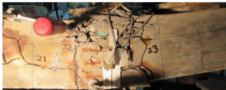
Figure 3.46 Formation of cracks during bending test of B38M-FS-16/160
