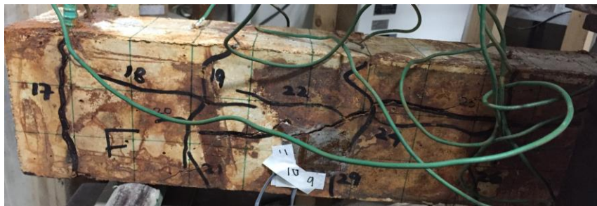
Figure 3.39 Formation of shear crack during bending test of B11S-FS-10/120
