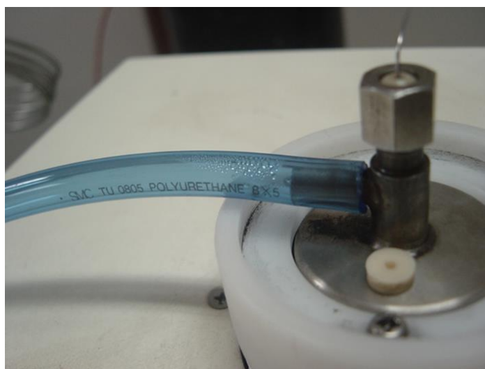
Figure 6-4: Water condensation during temperature stabilizing process by introducing N_2 gas
