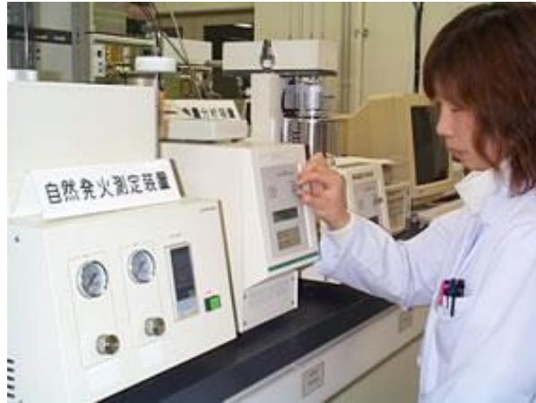
Figure 4-3: SHIMAZU Ignition Tester (SIT-2) at Idemitsu Co. to determine T_{180} value ( http://www.idemitsu.co.jp/rd/laboratory/environment/natural.html )
