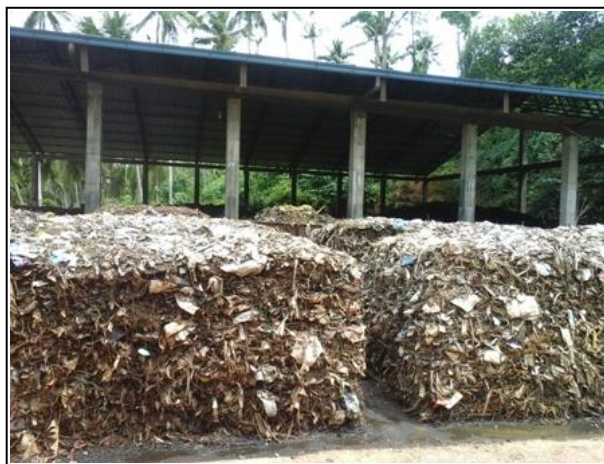
Figure 2- 6 Rectangular block type windrow piles in one visited facility
