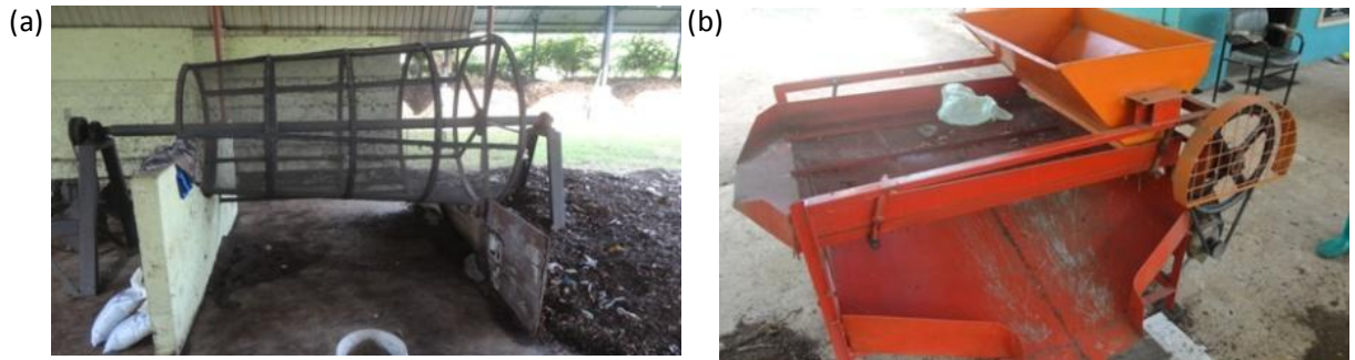
Figure 2- 17 Screening methods used by visited composting facilities (a) A trammel screening, (b) A vibrating table screening
