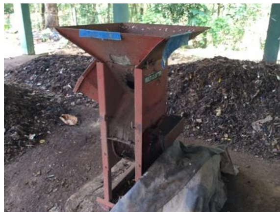
Figure 2- 19 A hammer mill type crusher used for reducing the coarse compost particles in residue
