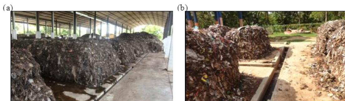
Figure 2- 8 Type of composting (a) Piles under a roof, (b) Piles without a roof- open composting
