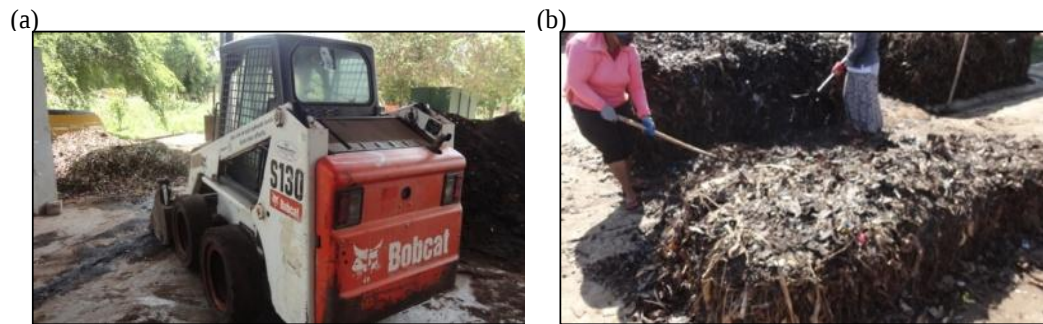
Figure 2- 11 Composting piles turning methods (a) turning mechanically using front wheel skid loaders (bob cats), (b) turning manually using shovels
