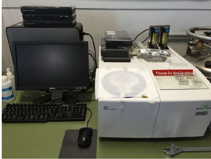
Figure 2.4. The photo of the Mettler Toledo DSC1 STAR c system (NIMS).
