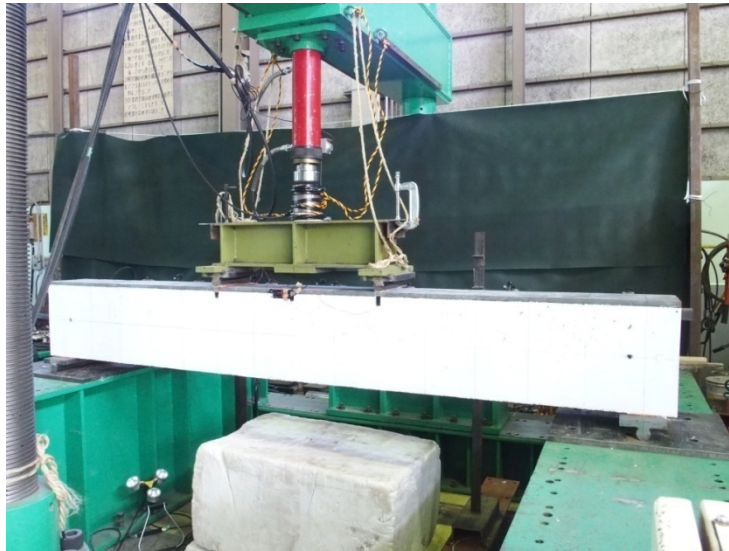
Figure 4: Flexural test setup
